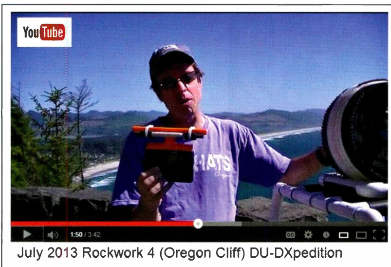
Photo A. Gary DeBock sets up his latest creation — a 22-pound, 12-inch diameter FSL antenna — at the Oregon cliff DXpedition site in this YouTube video. Watch and listen at < http://bit.ly/14xGtuj >. ( Internet screen grab )
