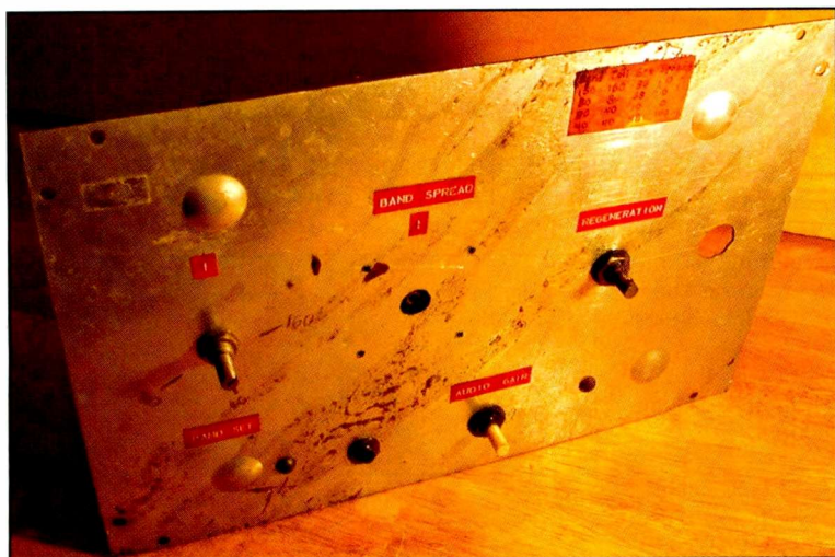
Photo A. It is clear to see that our "Little Electrical Disaster Survivor" has succumbed to time, scavenger, and the perils of Pop's radio sanctum since it was built six years ago. In happier times, the front panel was a thing of regenerative beauty with the band-set capacitor control on the left. In the middle, you can see the four holes where a nice vernier drive was mounted for band-spread tuning. The regeneration control was at the right and audio at the bottom. To the left of the audio was the headphone jack and the gaping hole on the upper right was where Pop and I put a pilot light — to remind me not to reach behind the front panel when the power was on. We made a little chart of capacitor settings and glued it near the top of the panel for easy reference. I'm not sure what that gunk is that dripped down the regen's face. It could be just about anything, given the rather "untamed" condition Pop's radio workshop was in. (Photography courtesy of KPC6KPH)
