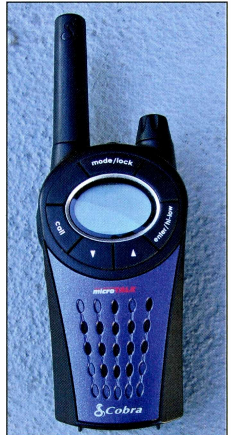
Photo A. Cobra’s Micro-Talk series of handhelds are GMRS-capable radios, < https://cobra.com >. (Courtesy of Wikimedia Commons)
