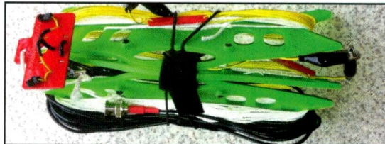
Photo C. SOTabeams newest High Hopper is a linked dipole that operates on the 20-, 17-, and 15-meter bands. (Courtesy of SOTabeams)
